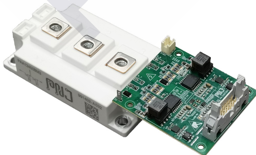
Fig. 1. 62mm half-bridge SiC module PAA12400BM3 and PNDM12P204A1
